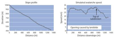
FIGURE 93 Deterministic application of the PCM avalanche dynamics model to the area shown in Figure 91.
