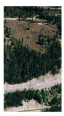
FIGURE 82 Avalanches initiating in the steep harvested terrain above the Trans-Canada Highway in the Kicking Horse Canyon have the potential to affect the highway even though the area is not often subject to deep snowpacks.
