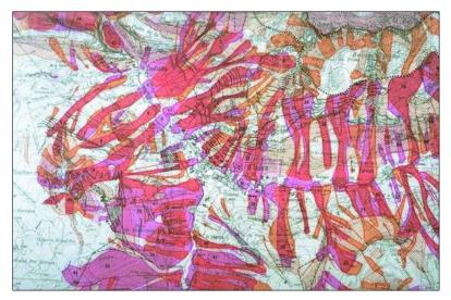
FIGURE 87 Avalanche mapping for Val d'Isère, France (scale 1:25 000). Mapping in orange is from air photo interpretation. Mapping in magenta is based on field surveys, interviews with local witnesses including Forest Service rangers, and ski patrollers. Solid cross-hatching implies more certainty than areas delineated with broken cross-hatching. (After Borrel 1992)
