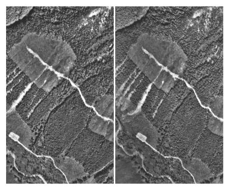
FIGURE 85 Stereopair of Nagle Creek avalanche path. A low-power pocket stereoscope is required to see the terrain in three dimensions. Scale approximately 1:15 000 (Airphotos 30 BCB97061 nos. 272 and 273).
