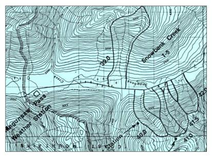
FIGURE 89 Ministry of Transportation avalanche mapping showing distribution of avalanche paths above highway at Ningusaw Pass, between Bob Quinn Lake and Stewart, B.C. (scale: 1:78 125). (No indication of frequency or maximum runout distance implied.)
