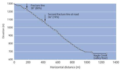
FIGURE 86 Slope profile of the Nagle Creek avalanche path plotted from 20-m TRIM contours.
