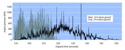
FIGURE 95b Impact pressures measured at two heights on a tower located in the path shown above. At 3 m above the ground quasi-static pressures were around 500 kPa for 30 seconds, with distinct peaks of up to 1200 kPa. (Dufour et al. 2000)
