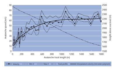
FIGURE 95a Radar speed measurements of the frontal pulse of a large avalanche gave a maximum of 80 m/s (290 kph) (dashed lines indicate error ranges associated with the measurements). The path falls 900 m. (Dufour et al. 2000)
