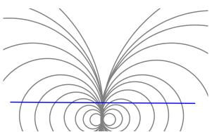
Figure 2a: The flux lines in the Vertical Plane of a vertical burial look like flux lines being sprayed up and out like a fountain. Following flux lines puts you right on top of the buried beacon.
