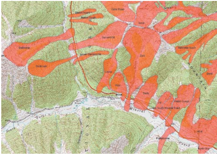
Avalanche-path mapping of the San Juan Mountains along US Highway 550 assist Colorado Department of Transportation (CDOT) road-maintenance workers. Highlighted red areas indicate the slide paths, making it easy to track and identify avalanche activity. Use of the GIS system is also a powerful budgetary tool, allowing CDOT to track avalanche control work by path and facilitating cost analysis on amount of explosives used, man hours and equipment wear and tear. For more about the history of avalanche control efforts along this particular stretch of road, see Red Mountain Pass – Chief Ouray Highway: A History of Forecasting and Mitigation , beginning on page 24.
